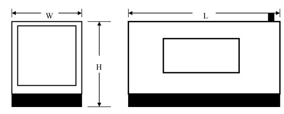
Dimensions are subject to change. Please consult your sales rep for proper sizing. Proper concrete slab size should be 3 feet larger on each size for ease of maintenance.
